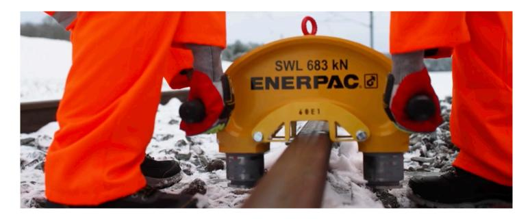
Rail stressors are vital tools used to pull and tension railway tracks during maintenance, repair, and construction. Common applications include closing gaps in preparation for thermite welding and adjusting the tension in Continuous Welded Rail (CWR) to prevent deformations caused by changing environmental conditions.
