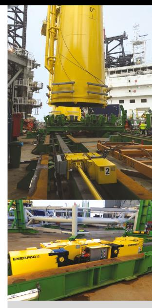
**PRODUCTS** Enerpac ETR50, ETR100 and ETW125 electrically driven trolley systems
