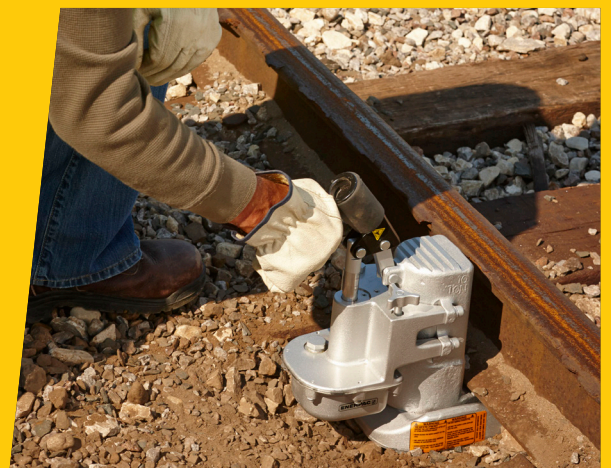
Handle on the TJ-Series Jack can be used at the first stage to advance the toe until resistance is felt.
