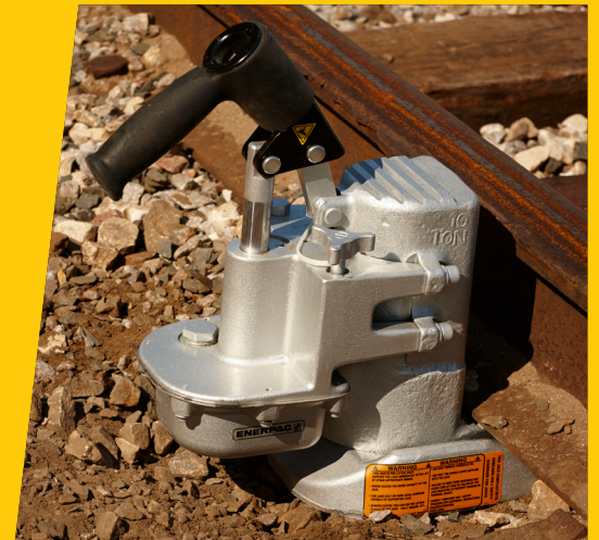
TJ-Series Track Jack with toe positioned under the track.
