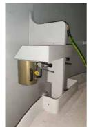
Six to twelve pre-installed hydraulic cylinders inside the TP make it possible to align the TP to a precise position, even if the MP was not completely levelled out in the first place. This ensures that the turbine will generate maximum yield.
