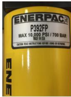
FIGURE 15 LABEL FOR AFTERMARKET PARTS ON THE PART ITSELF.
