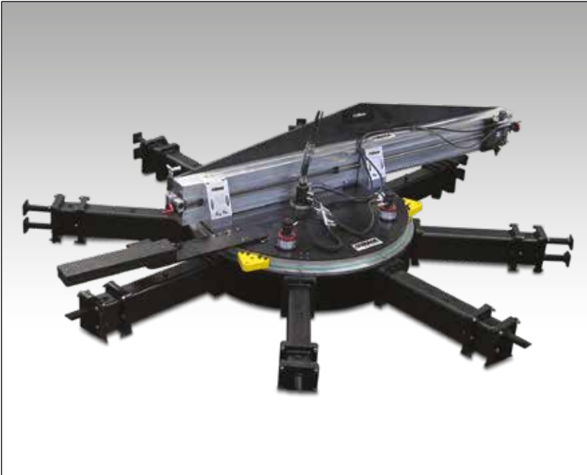
▼ OM6000 Orbital Milling Machine
