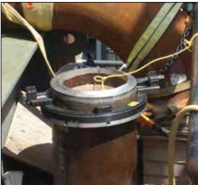
◀ NB-model narrow body clamshell cutter.
