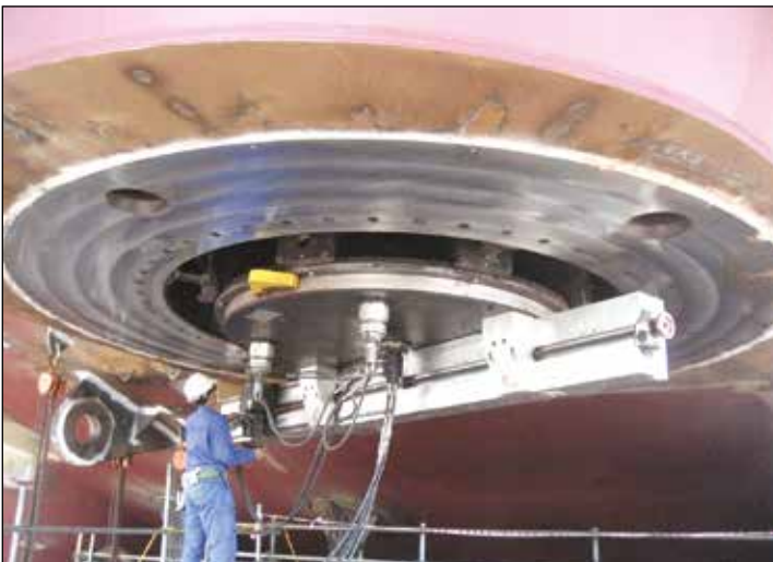
▼ Milling a ship thruster flange.
