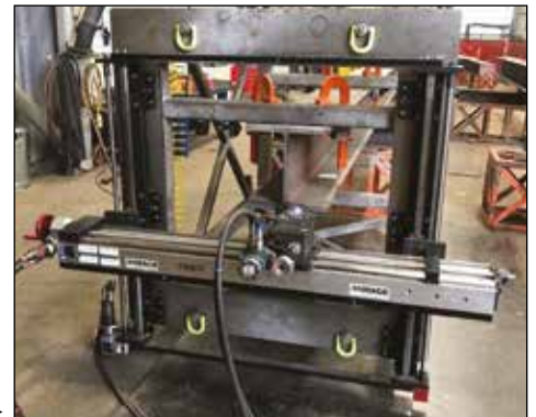
I-Beam end face milling with a GMRF1000. ▶
