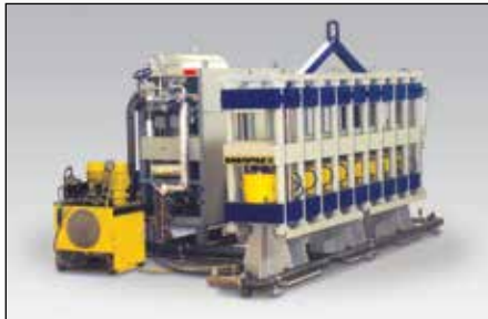
◀ Fully Automated PLC-Controlled 1800-Ton, High-Accuracy Press
