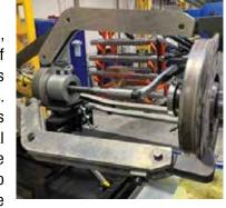
handling to prevent safety incidents and component damage. Unlike practices such as torching and hammering, using purposedesigned hydraulic pulling equipment ensures a safe removal process and avoids expensive damage to components. Using a 100-ton capacity puller mounted onto a stable trolley can allow a single operator to remove large wheels and bearings efficiently, and safely captures removed components.
