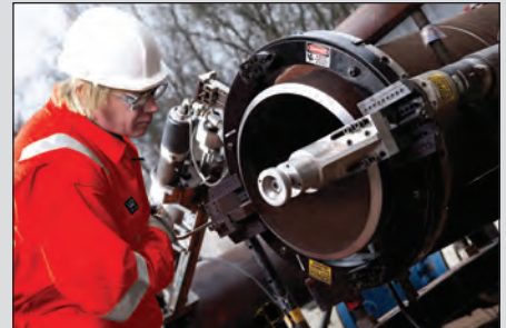
▲ Pipe cutters and weld preparation.
