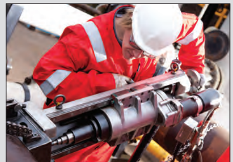
▲ High torque portable drilling machines.
