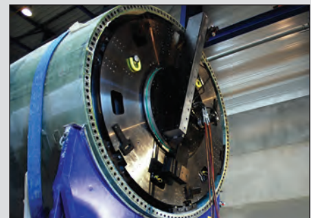
▲ Orbital milling machines for wind turbine manufacture.
