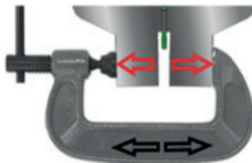
Fig. 4. Forces applied to G-Clamp during hot bolting operations
