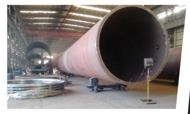
Tower sections and transition pieces are typically manufactured in a different facility to a blade manufacturing. Fabricators of these huge steel tower sections are also expected to deliver repeatable precision but also face different challenges to blade manufacturers.
